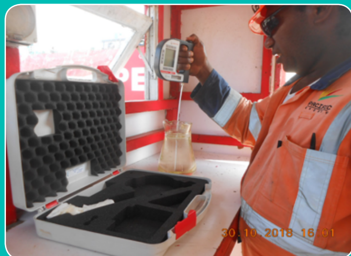
SSP staff taking readings for fuel quality parameters during fuel transfer from tanker to shore terminal storage tanks
